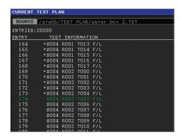
The MIZ-28 imports an inspection Test Plan and displays it for the operator.
